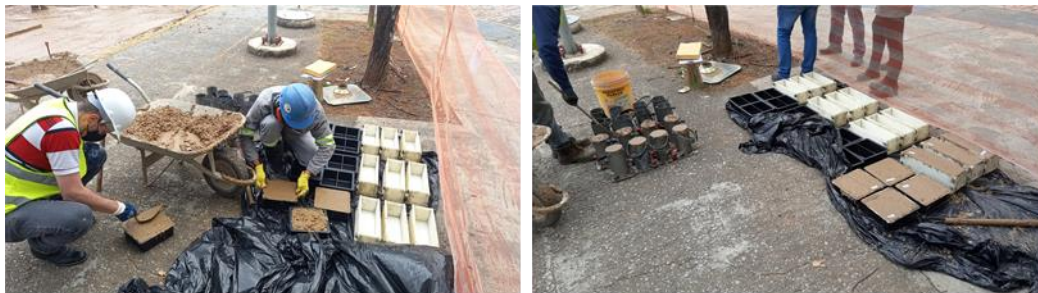
Figure 5. Preparation of samples for the hardened state control of monolithic concrete.
